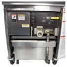
Designed to complete a filter cycle in 5 minutes. System uses disposable paper media and basically allows 1-step draining, filtering, and vat cleaning. Turn a single valve to refill vat with
