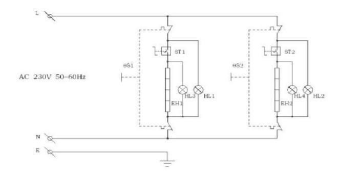
QS1 QS2 Temperature limiter EH1 EH2 Heating Element
