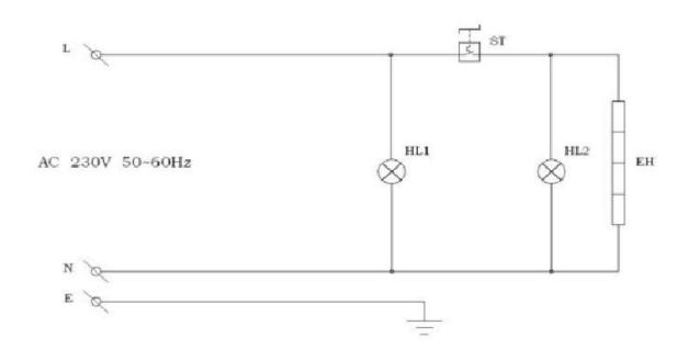
QS Temperature limiter EH Heating Element ST Thermostat
